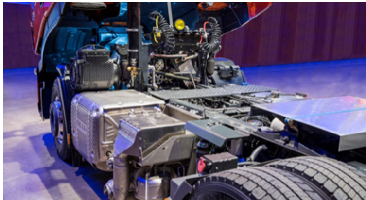
Figure 1.1: The prototype of a waste heat recovery ORC-system on board of a long-haul truck. Courtesy of AVL GmbH.
