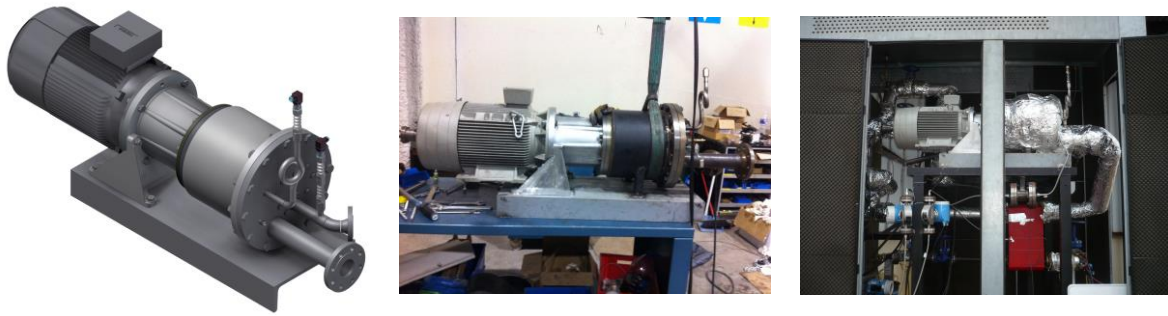
Figure 3: Simulated and constructed prototype and the ORC test bench
