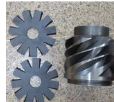
Figure 2: Main rotor and gate rotor
