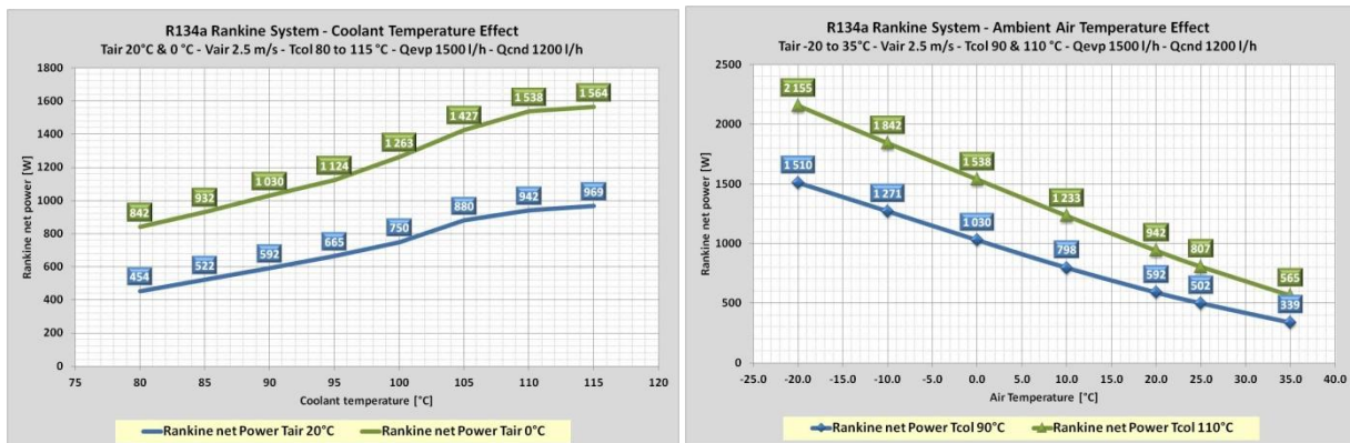
Figure 5 : Effect of operating conditions on optimal Rankine system performance a: HT coolant temperature effect b: Ambient air temperature effect
