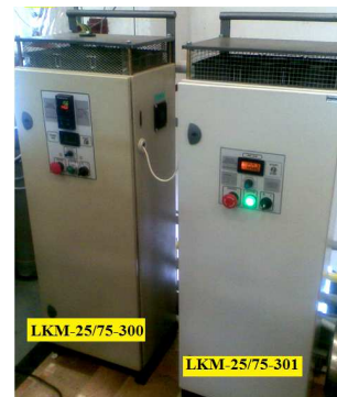
Figure 5: Prototype electric flow heater for thermal oil
