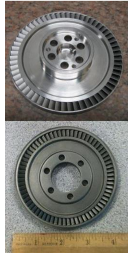
Finished Machined Rotor (one of three used in the CN300 system)
