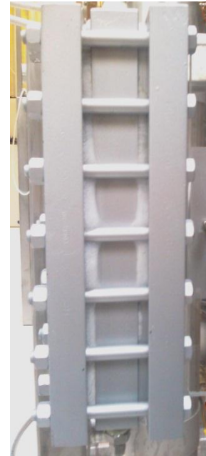
Brazed plate HX with bolted frame
