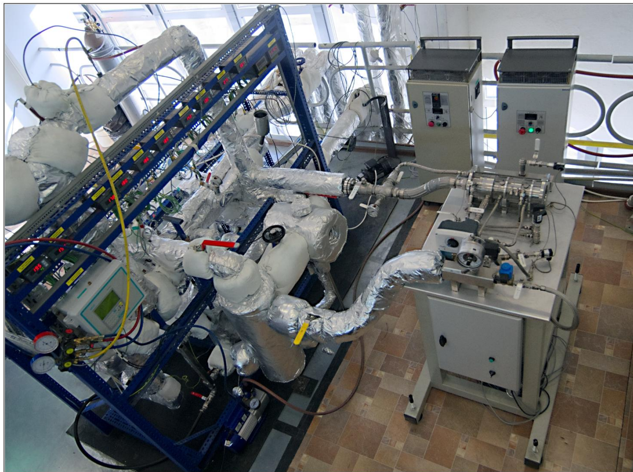
The ORC system with a microturbine and a set of heaters in the test bench in the Institute of Fluid-Flow Machinery of the Polish Academy of Science in Gdańsk.
