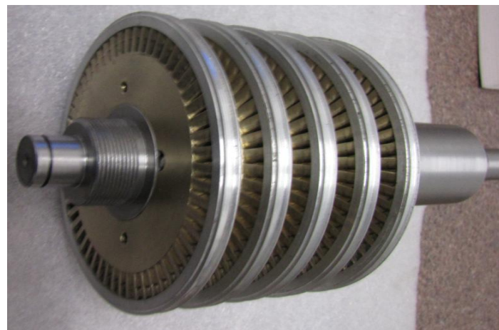
Shrouded rotor of a axial turbine.
