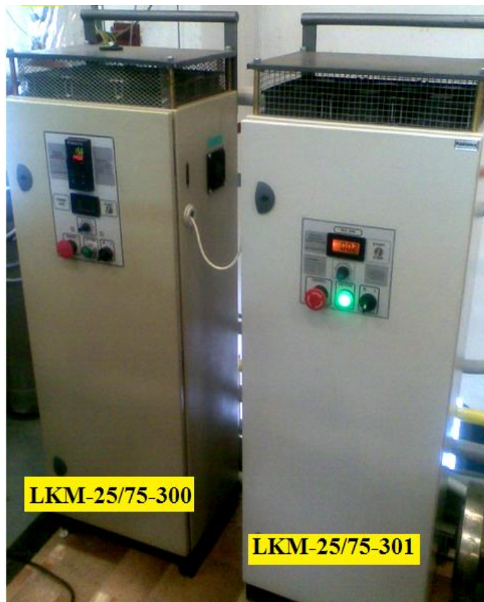
Prototype of electric flow heater for oil.
