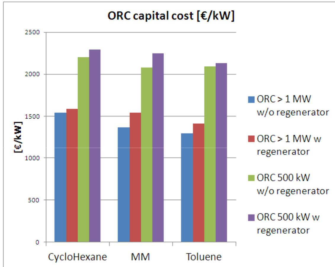
Although the net power obtained with cyclohexane is greater than that of the other working mediums, the specific cost of the plant implementing such a fluid is the highest. This is due to the high evaporation pressure of the cycle.
