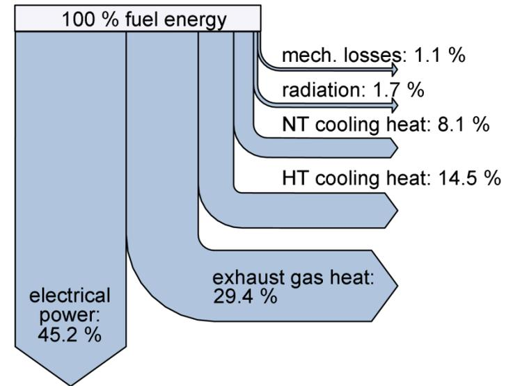
Heat flux diagram of state of the art internal combustion engine
