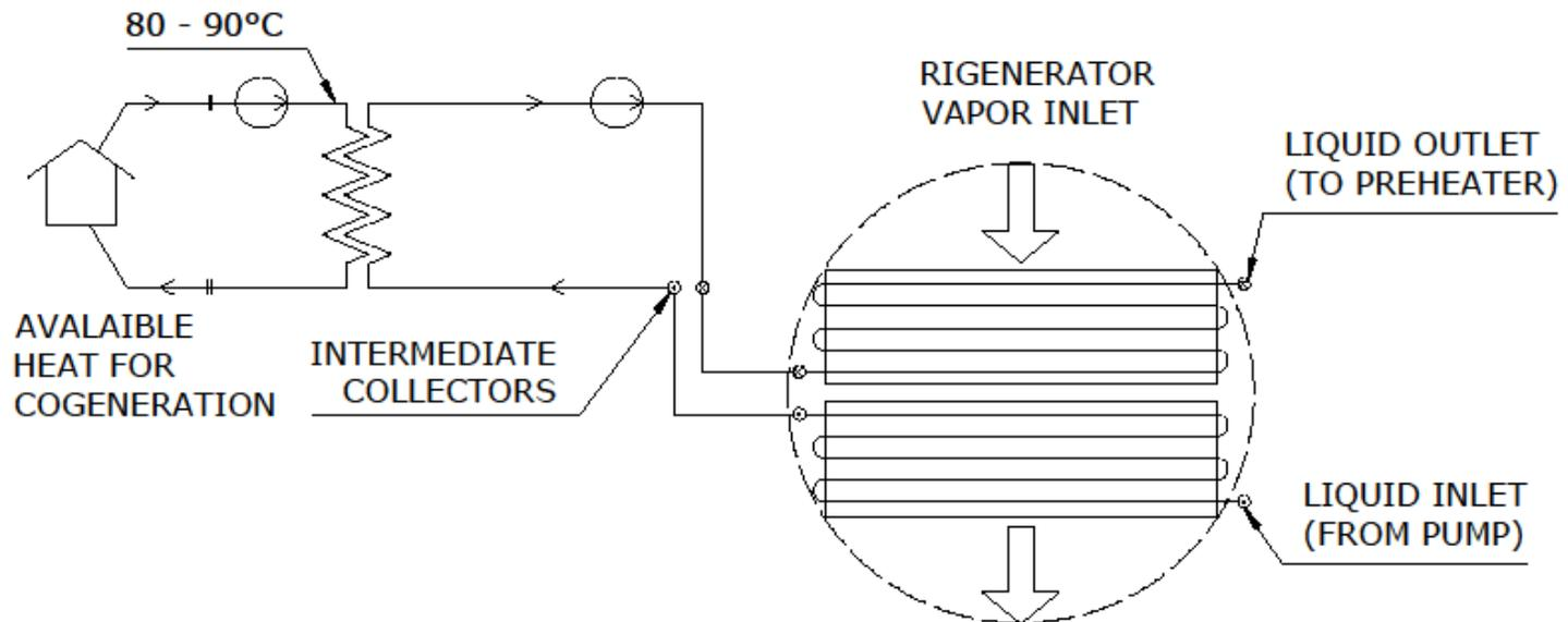
⇒ The additional circuit allows to utilize a fraction of the heat available in the regenerator to heat up a flow of water at a temperature higher than condenser temperature
