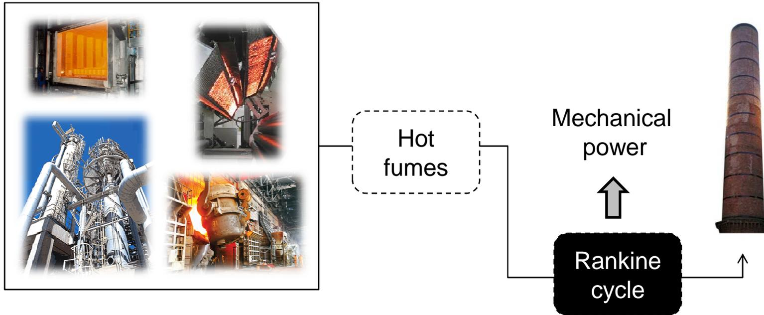
**The heat that is not transferred to the ORC is released to the atmosphere.**
