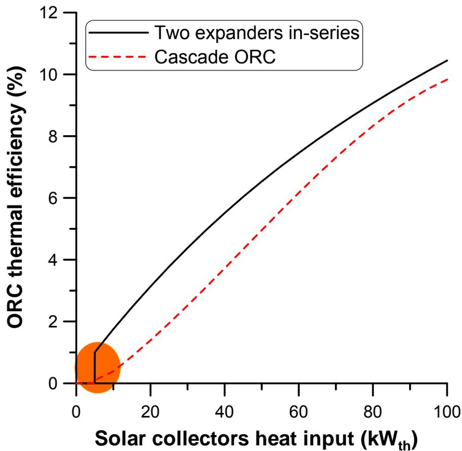
The system operation is stopped, when the collectors' heat gain is lower than 5 kW<sub>th</sub> (ORC evaporation temperature ~50 °C, according to a pinch point analysis)
