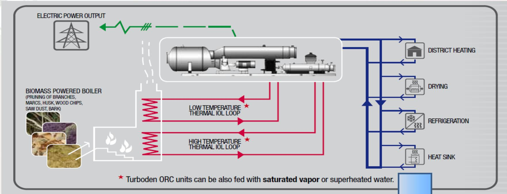
In cogeneration systems, water temperature at the condenser output is high enough to satisfy heat consumers, but low enough not to penalize too much ORC efficiency
