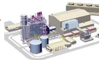
Waste Heat Bottoming Cycle to a Gas Turbine
